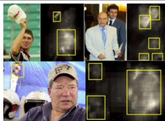
Figure 4: CNN Face detection. This image shows the potential faces found by the CNN after one pass through (Yang & Nevatia, 2016)
