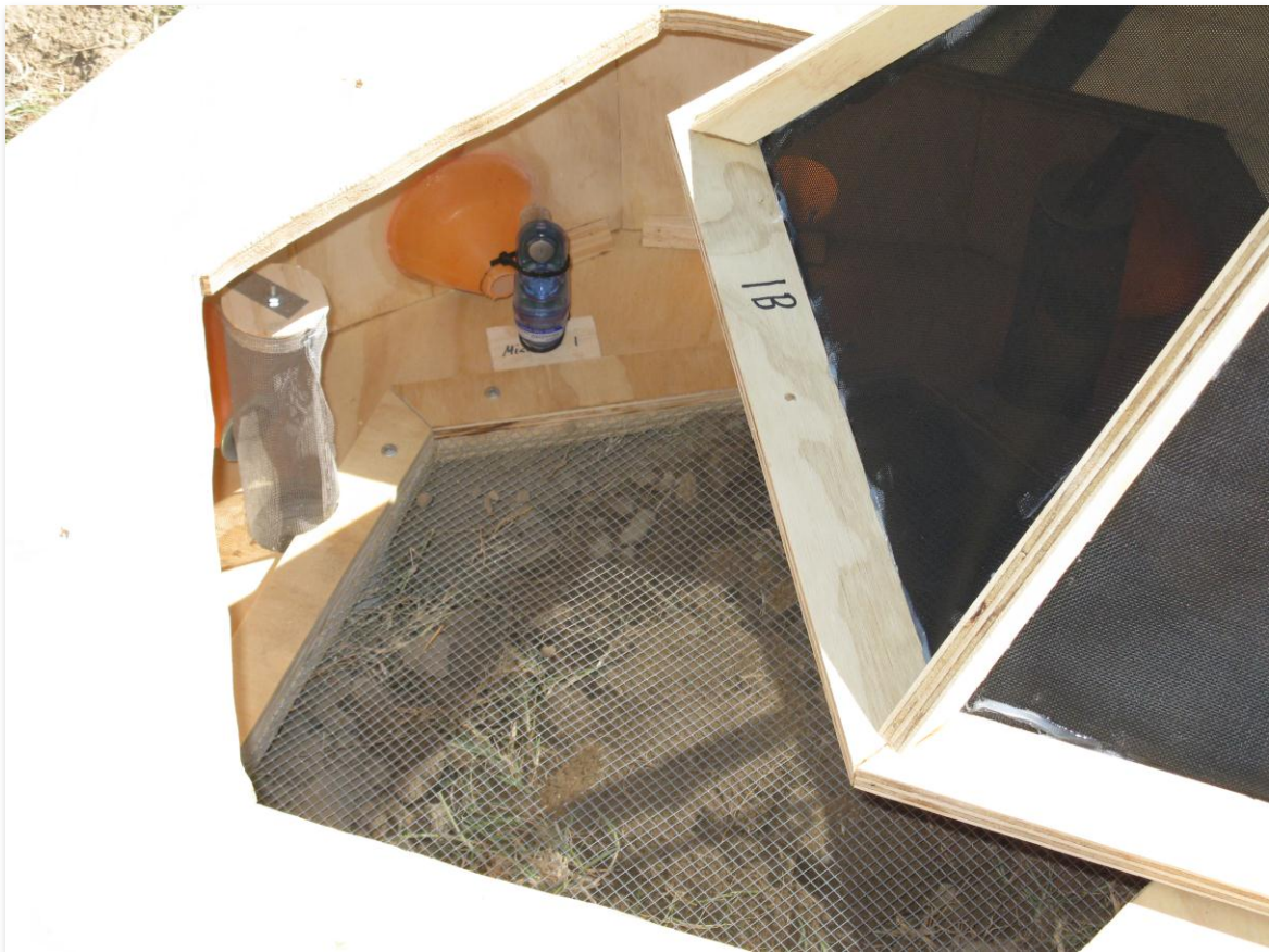
Picture 6. Interior Temperature/Moisture Data Collector.
