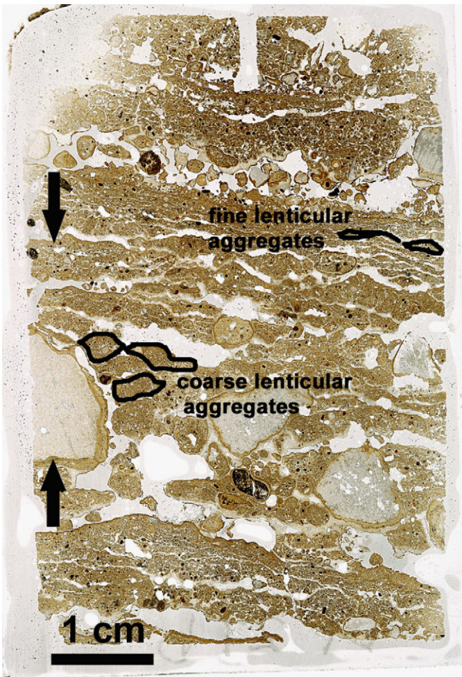
Fig. 17. Photograph of a thin section from layer I showing an increment (between arrows) with decreasing size of ice lensing upwards.
